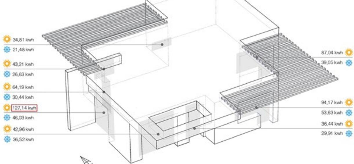
04 | Simulations for the optimization of the relationship between the shape of the building and the levels of natural lighting and reduction of the thermal load on the transparent envelope
