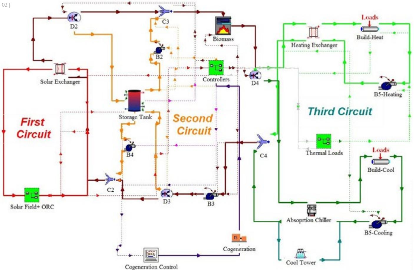
02 | Thermal polygeneration plant for a district area modelled in TRNSYS
